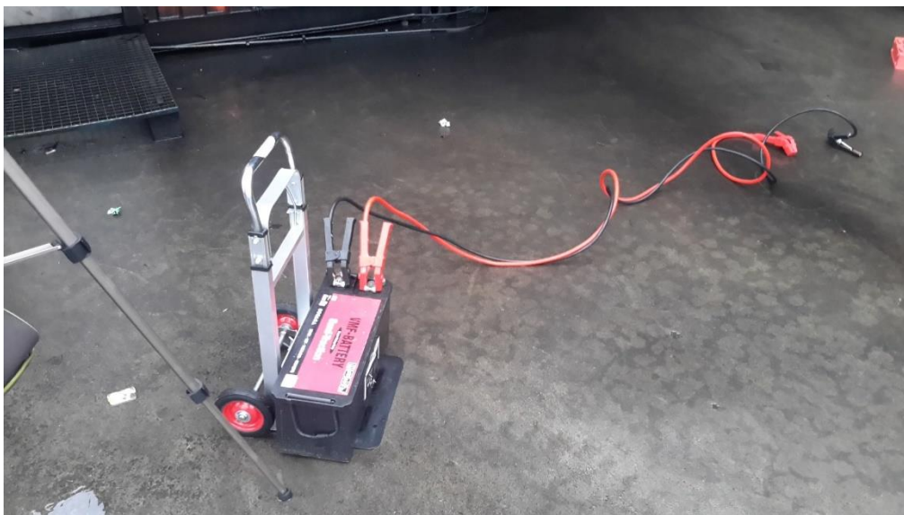
Battery for the activation of the glow plug
